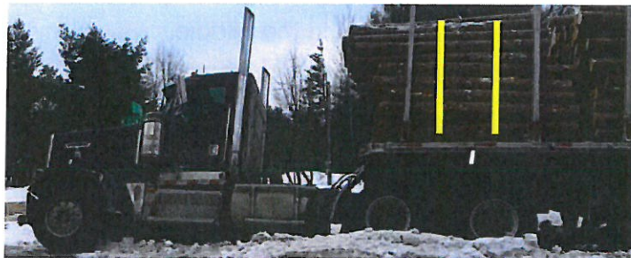
Two Tiedowns Required Over Front Stack for Driver Protection
